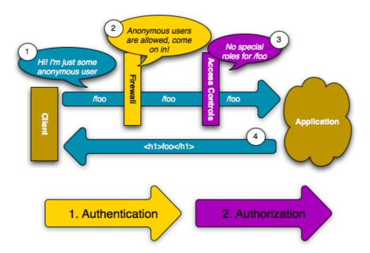
This works first because the firewall allows *anonymous users* via the **anonymous** configuration parameter. In other words, the firewall doesn't require the user to fully authenticate immediately. And because no special **role** is needed to access **/foo** (under the **access\_control** section), the request can be fulfilled without ever asking the user to authenticate.
