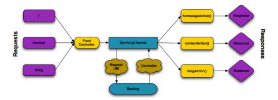
The routing layer is a tool that translates the incoming URL into a specific controller to execute.
