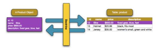
For Doctrine to be able to do this, you just have to create "metadata", or configuration that tells Doctrine exactly how the Product class and its properties should be *mapped* to the database. This metadata can be specified in a number of different formats including YAML, XML or directly inside the Product class via annotations:
